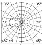
Luminous flux luminaire 580 lm
