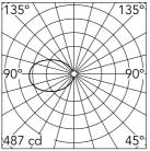
Luminous flux luminaire 551 lm
