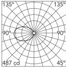
Luminous flux luminaire 580 lm
