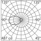
Luminous flux luminaire 551 lm
