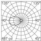
Luminous flux luminaire 551 lm
