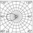
Luminous flux luminaire 551 lm
