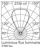
Beam Angle: 63° h(m) E(Ix) D(m) 2336 1.23 1 2.46 2 584 3 260 3.69 146 4.92 4 5 93 6.15
