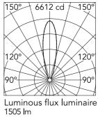
Beam Angle: 25° h(m) E(Ix) D(m) 6612 0.45 1 0.90 2 1653 1.35 3 735 1.80 4 413 5 2.25 264
