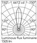
Beam Angle: 25° h(m) E(Ix) D(m) 6612 0.45 1 0.90 2 1653 1.35 3 735 1.80 4 413 5 2.25 264
