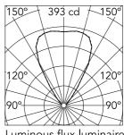
Luminous flux luminaire 414 lm
