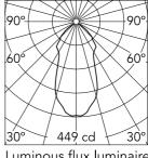
Luminous flux luminaire 483 lm
