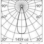
Luminous flux luminaire 468 lm (EXTREME CUT OFF)
