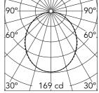
Luminous flux luminaire 446 lm
