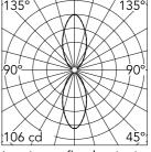
Luminous flux luminaire 164 lm
