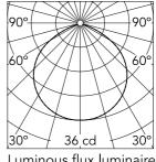
Luminous flux luminaire 96 lm
