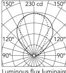
Luminous flux luminaire 407 lm
