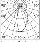
Luminous flux luminaire 2116 lm
