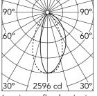
Luminous flux luminaire 2560 lm
