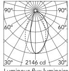
Luminous flux luminaire 2116 lm
