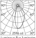
Luminous flux luminaire 2560 lm
