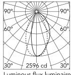
Luminous flux luminaire 2560 lm
