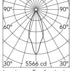
37° Beam Angle: h(m) = E(Ix)D(m) 5566 0.67 1.34 1392 3 618 2.01 348 2.69 5 223 3.36
