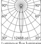
Luminous flux luminaire 1648 lm
