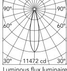
24° Beam Angle: h(m) = E(Ix)D(m) 11472 0.43 2 2868 0.86 3 1275 1.28 4 717 1.71 5 459 2.14
