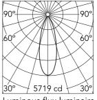
Luminous flux luminaire 1947 lm
