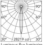
Luminous flux luminaire 2190 lm
