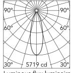
Luminous flux luminaire 1947 lm
