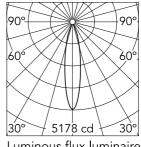
Luminous flux luminaire 941 lm
