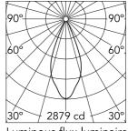
Luminous flux luminaire 1216 lm
