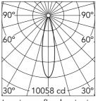
Luminous flux luminaire 2134 lm
