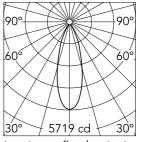
Luminous flux luminaire 1947 lm
