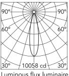
Luminous flux luminaire 2134 lm
