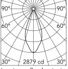
Luminous flux luminaire 1216 lm
