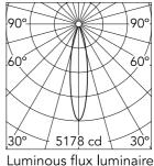
21° Beam Angle: h(m) = E(Ix)D(m) 5178 0.37 0.73 2 1294 3 575 1.10 4 324 1.47 5 207 1.83
