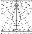
Luminous flux luminaire 1216 lm
