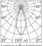
Luminous flux luminaire 1394 lm
