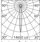
Luminous flux luminaire 1255 lm
