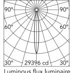
Luminous flux luminaire 2281 lm
