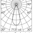
Luminous flux luminaire 2644 lm
