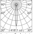
Luminous flux luminaire 3664 lm
