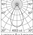
Luminous flux luminaire 2986 lm
