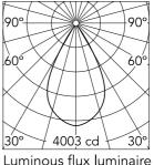
Luminous flux luminaire 2986 lm
