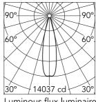
Luminous flux luminaire 2895 lm
