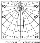
Luminous flux luminaire 3637 lm
