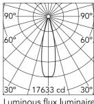
Luminous flux luminaire 3637 lm
