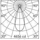
Luminous flux luminaire 1838 lm
