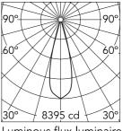
Luminous flux luminaire 1816 lm
