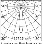
Luminous flux luminaire 1872 lm
