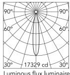
Luminous flux luminaire 1872 lm
