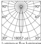
Luminous flux luminaire 1951 lm
